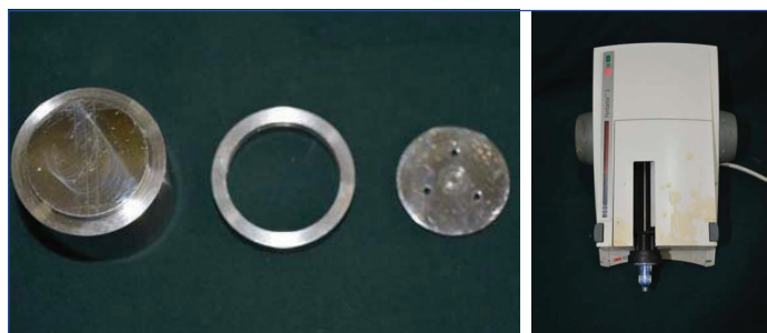
[Table/Fig-2]: Die fabrication (according to ADA specification no. 19). [Table/Fig-3]: Pentamix machine. (Images from left to right)
