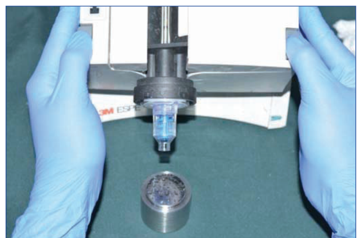
[Table/Fig-10]: Impression procedure for vinyl siloxane ether under moist condition.
